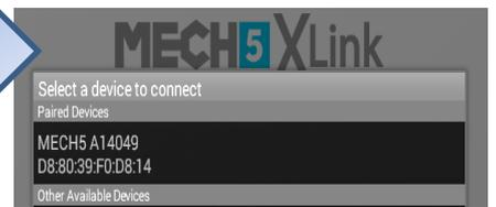
**HELP TIP:** If you are unable to connect to the device. Unplug your VCI from the vehicle OBD port and then reconnect it. Then, go to your Android device Bluetooth settings to add the VCI manually.
